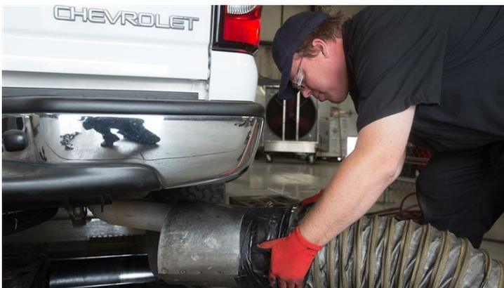
*Charles Eckersell hooks an exhaust hose to the tailpipe of a diesel pickup truck during an emissions test at the Davis County Testing Center on Thursday, Aug. 25, 2016. All diesel vehicles in Davis County are required to have an emissions test, similar to gasoline powered vehicles.
