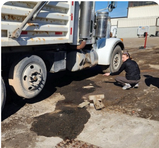
A licensed environmental health scientist investigates a fuel leak impacting a storm drain.
